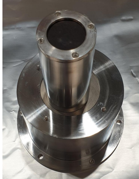
(b) The cup before installation with the adjustable insert and the Be foil.
